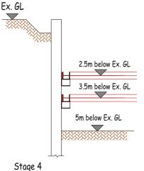
Excavate to formation level, 5m below existing ground level
