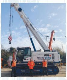
working within the railway environment such as HS2. It can easily lift our Kowan Stillworker Rigs that weigh circa 11 tonnes off the back of the delivery lorry. Fitted with a 30.4m jib as standard we can stand well back to lift long piles into position once the rig is set up and progressing.
