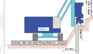
Max Rectangular Bearing Pressure = 430 kN/m2 Equivalent track bearing length = 2.33m Track width = 0.7m (Load Case 2 Extracting with Auger )
